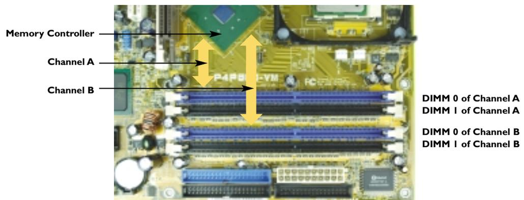
For the best dual-channel memory performance on motherboards with the Intel dual-channel DDR chipsets, you must use identically paired memory modules in DIMM sockets 0 of channel A and B. Identically paired memory modules must also be used when populating DIMM sockets 1 of channel A and B. One can, for example, plug in matching 256MB DIMMs in both DIMM 0 slots, and plug in matching 512MB DIMMs in both DIMM 1 slots.
