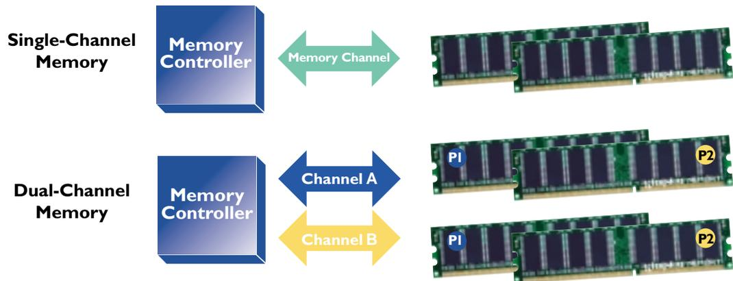
With dual-channel memory, the memory controller is able to move double the peak amount of data that it could normally move with single-channel memory. That's because it is sending or receiving data from two memory module pairs at the same time (shown as module pairs "P1" and "P2" in the graphic above).
