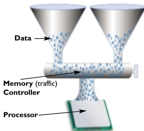
same way when data is “emptied” from the processor by reversing the flow of data. To prevent the funnel from being over-filled with data or to reverse the flow of data through the funnel, there is a “traffic” controller shown as a valve on the funnel's pipe. In computers, there is a special chip called the “Memory Controller” that handles all data transfers involving the memory modules and the processor.
