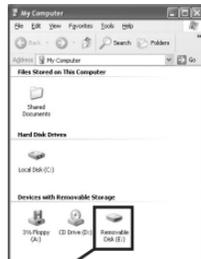
A new drive letter will be created for the card that can be accessed via the My Computer utility. Transferring files to and from the card is a simple drag-and-drop operation.
